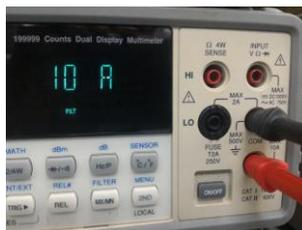
12. Rotate the knob to **CAL C** to calibrate output current.
